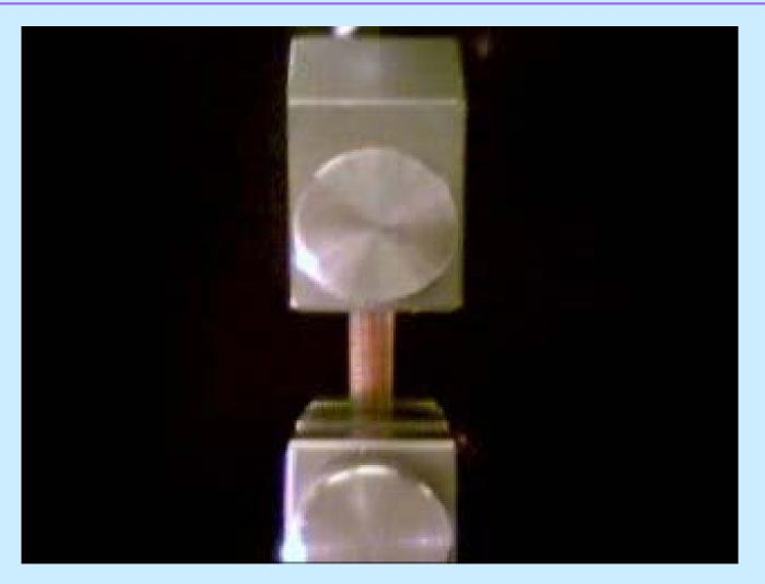
15 x 5 x 0.7 mm 500mm/min 100% strain 5 cycles
